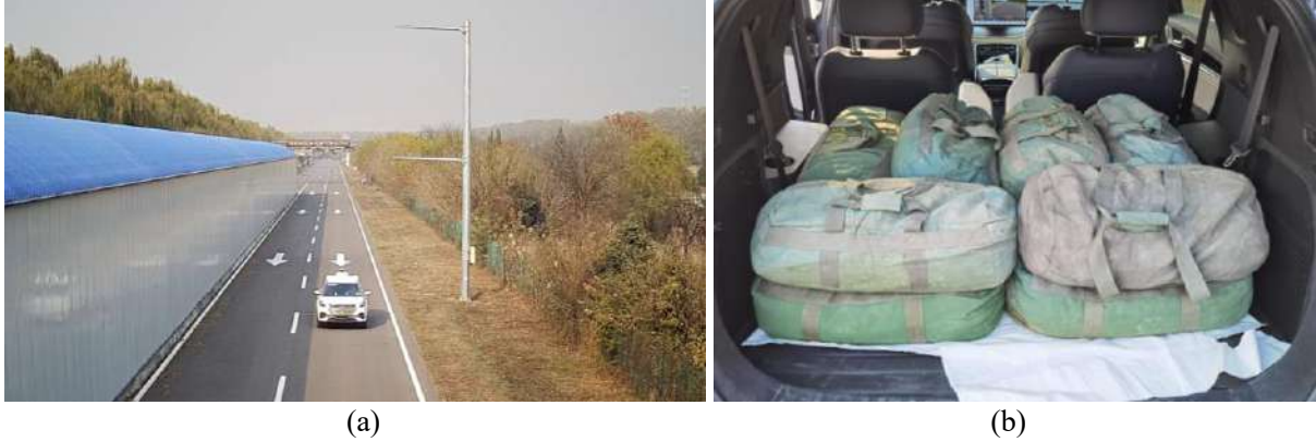
Figure 1. Snapshot of the experiment. (a) The AV tracking the pre-specified speed. (b) The load applied using standard sandbags, each weighing 25 kg.
